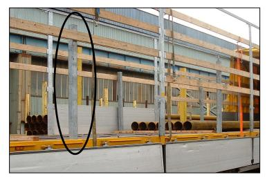
when open trailers are allowed, the load must be protected against the weather conditions by using covering sheets. Covering of the load needs to be done as safely as possible. The risk of falling from height should be prevented by taking adequate pro-active measures. Follow the specific local site regulations. The covering sheets must be undamaged, not porous and must be dry. Their surface must cover the entire load.
